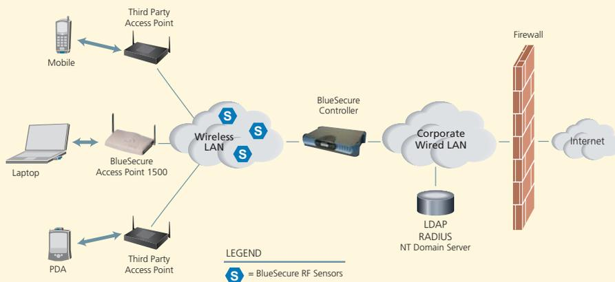
The BlueSecure Controller acts as a firewall between the wireless LAN access points and the wired LAN, and requires no changes to existing wired LAN hardware or user client software. Additional BlueSecure Controllers can be connected to provide hot failover capability, as well as scalability and subnet mobility across the enterprise.
